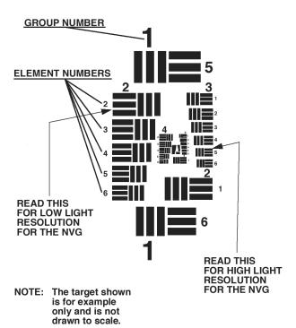
Figure 2-2. TS-4348/UV Test Set Pattern.
